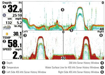
**Classic layout:** The top portion of the display presents a historical log of sonar returns from the 200 kHz down-looking sonar beam. New information in the down beam panel scrolls from right to left. The bottom portion of the display presents a historical log of sonar returns from the 455 kHz right- and left-looking sonar beams. New information appears at the top and scrolls down the display.
